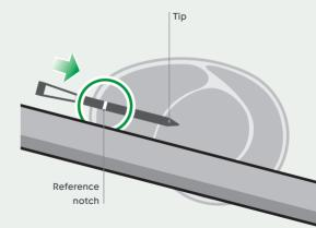
To use Thermomix® Sensor, fish or meat fillets should not be less than 3⁄4 in. (2 cm) thick.
