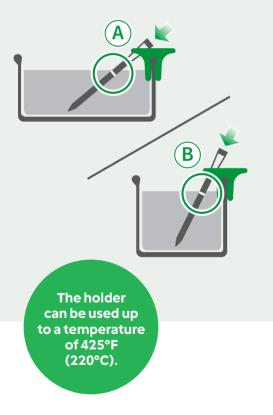
Place the holder on the edge of the baking pan as shown below, slide the probe through the holder then into the food.
