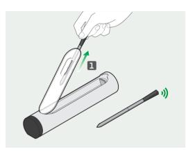
**4.** Open the charger and extract the probe. When you remove the probe from the charger, the LED flashes green indicating the charger is connected to the probe.
